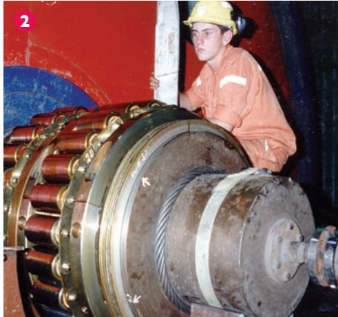
2. A 700mm diameter special double bearing supplied for a tower mounted winder in a copper mine. Normal operating load is 185 tonnes and the speed is 54 rpm.
