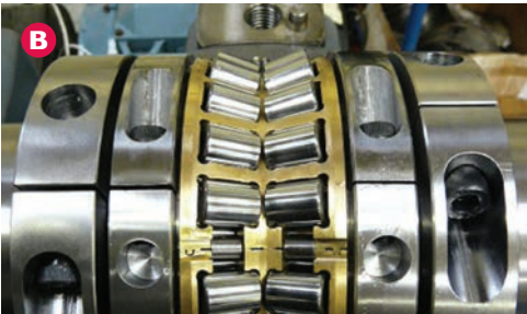
Cooper tapered roller bearing for marine Z-drive propulsion for intermittent thrust loading.
